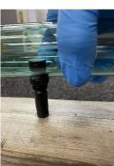
8. In the case of tight fitting, the hardware on the bottom end of the Tube can be secured to the wall with a shorter threaded rod
